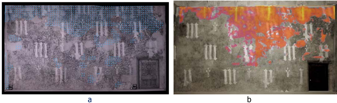
Comparison between the graphical representation of the mapping result obtained by knocking method (a) and detached zones identified by IRT on the west wall of dn (b). There is a good correspondence with the results of the manual knocking tests, especially in the upper part.
