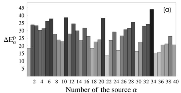
Figure 2. Colour distance (CIE Lab) of rock paint for 40 standard light sources regarding the torch.
