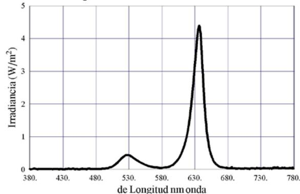
Figure 6. Spectral distribution of the proposed LED light source.
